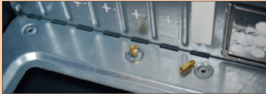
Figure 8-27 Spacers installed in case holes keep the motherboard from causing a short
