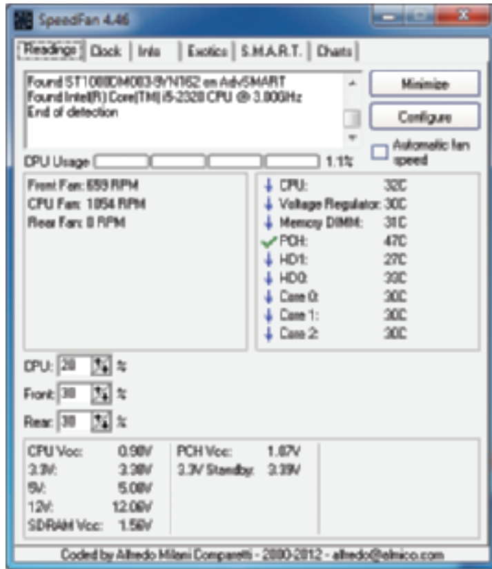
Figure 8-8 SpeedFan monitors fan speeds and system temperatures
