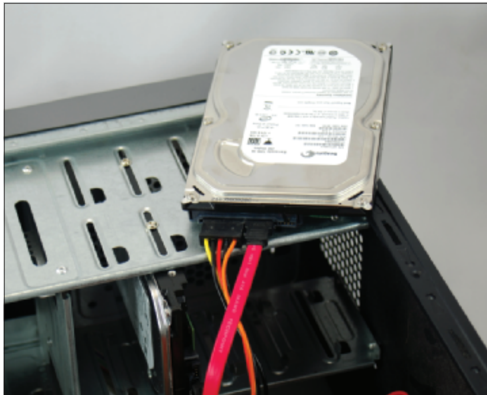
Figure 8-5 Move a hard drive to a working computer to recover data on the drive
