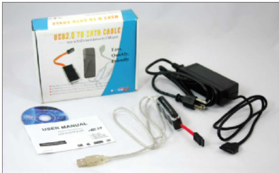
Figure 8-7 Use a USB-to-SATA converter to recover data from a drive using a SATA connector
