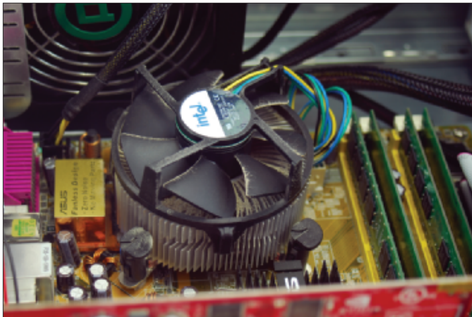
Figure 8-9 Dust in this cooler fan can cause the fan to fail and the processor to overheat
