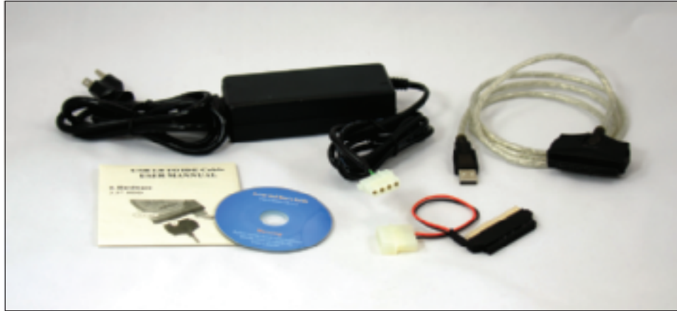
Figure 8-6 Use an IDE-to-USB converter for diagnostic testing and to recover data from a failing PATA hard drive
