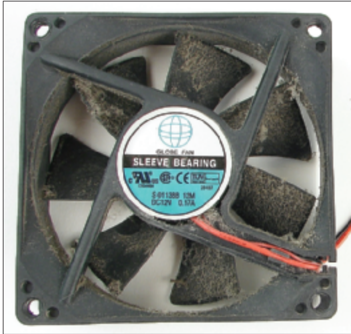
Figure 8-39 This dust-jammed case fan caused a system to overheat
