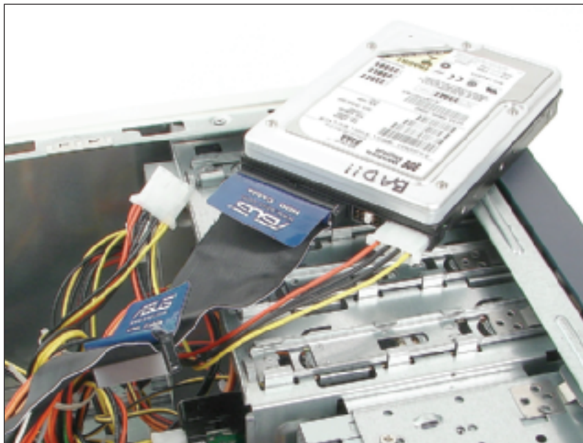
Figure 8-28 Temporarily connect a faulty hard drive to another system to diagnose the problem and try to recover data
