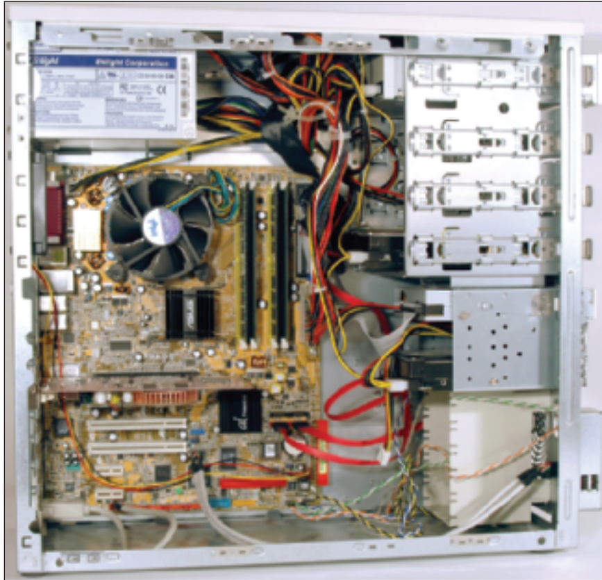
Figure 8-12 Use cable ties to hold cables out of the way of fans and airflow
